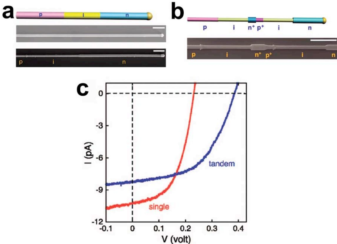
**Figure 1.** **a)** Schematic and SEM images of a single p-i-n SiNW. The bottom SEM image shows a single p-i-n SiNW after selective wet etching. Heavily doped n-type region is slowly etched, compared to the p- and i-type Si regions. **b)** Schematic and SEM images of a tandem p-i-n<sup>+</sup>-p<sup>+</sup>-i-n SiNW. **c)** Representative I-V curves of a single p-i-n SiNW and a tandem SiNW. Scale bars are 1  $\mu\text{m}$ .
