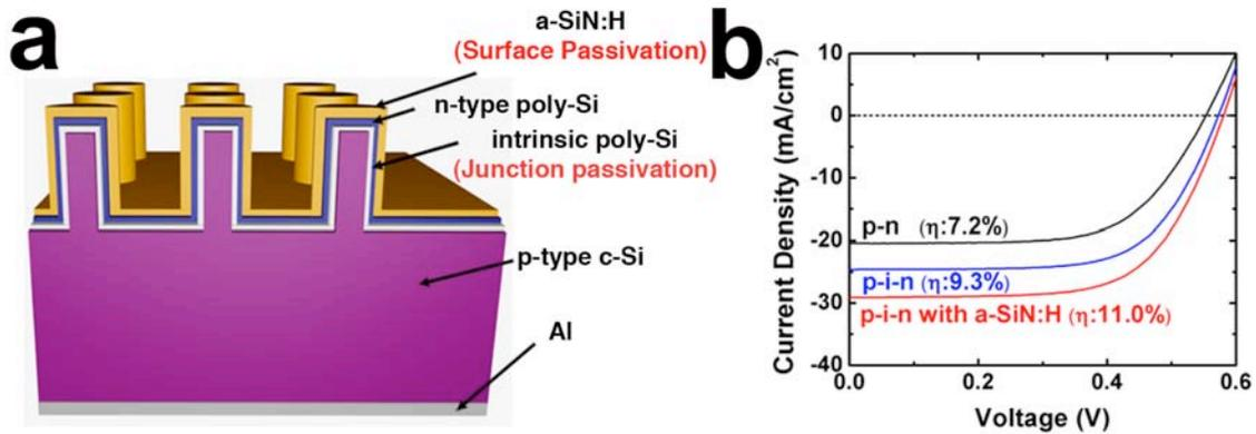
**Figure 3.** a) Schematic of a vertically aligned hybrid Si microwire (radial junction) and planar solar cell. b) Representative I-V curves of the hybrid solar cells, showing effective junction and surface passivations.
